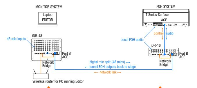
**Master system** The iDR-48 provides a large number of **mic inputs for sources on stage, and plenty of o**utputs to feed the wedge and IEM monitors.
